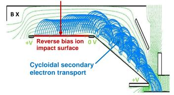
Transport of the electrons along the amplifying section is then optimised using a specialised ETP patented permeable grid [patent - WO2017132731A1].
